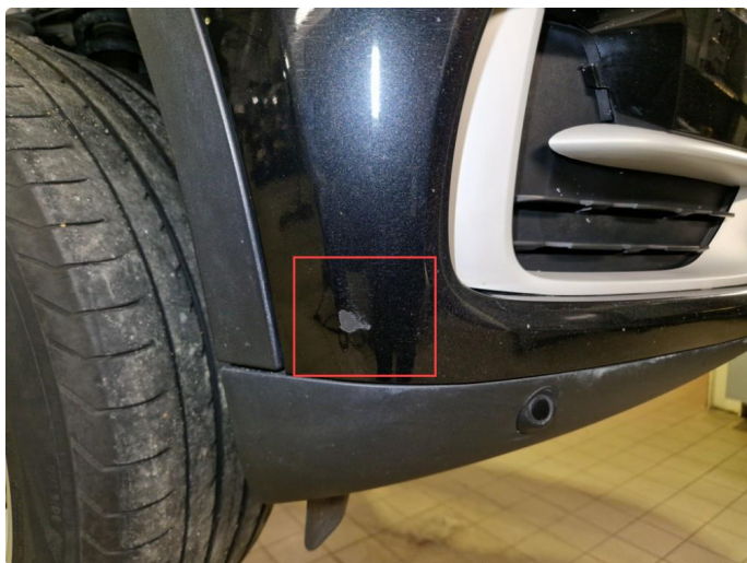
2.7 Lakkskader h-side frontfanger.
