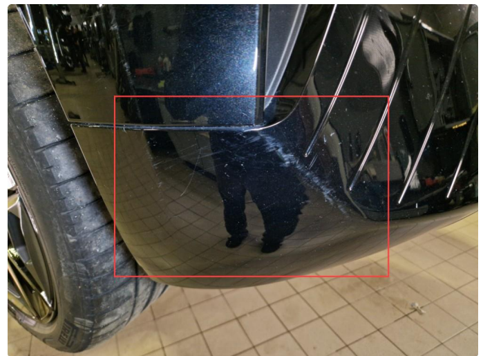
1.2 Noe riper h-side frontfanger .
