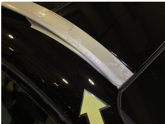
1.8 Noe lakkflask takrails.
