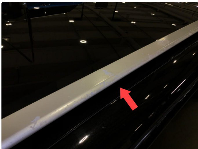
1.8 Noe lakkflask takrails.
