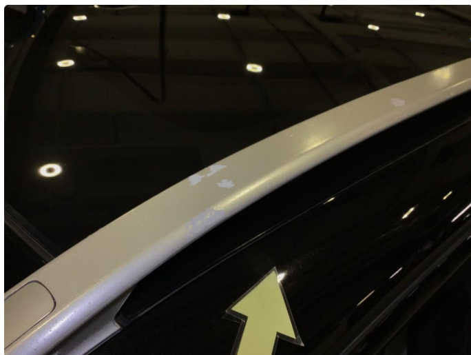
1.8 Noe lakkflask takrails.
