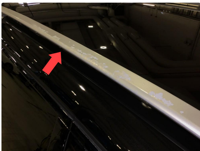
1.8 Noe lakkflask takrails.
