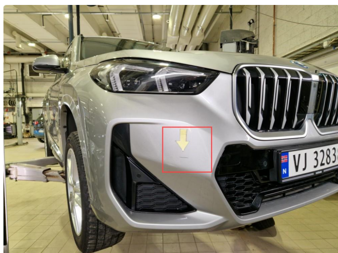
1.3 Ripe h-side frontfanger ( Poleres / Flekkes )
