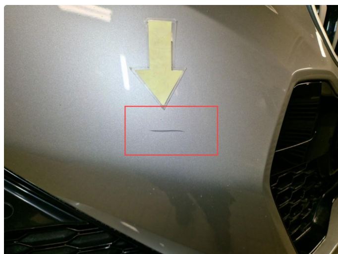
1.3 Ripe h-side frontfanger ( Poleres / Flekkes )
