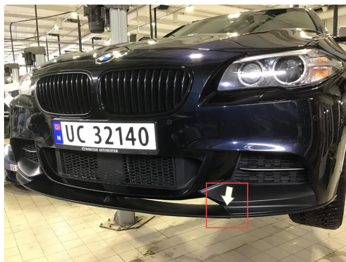
1.5 Liten sprekk i montert frontleppe.
