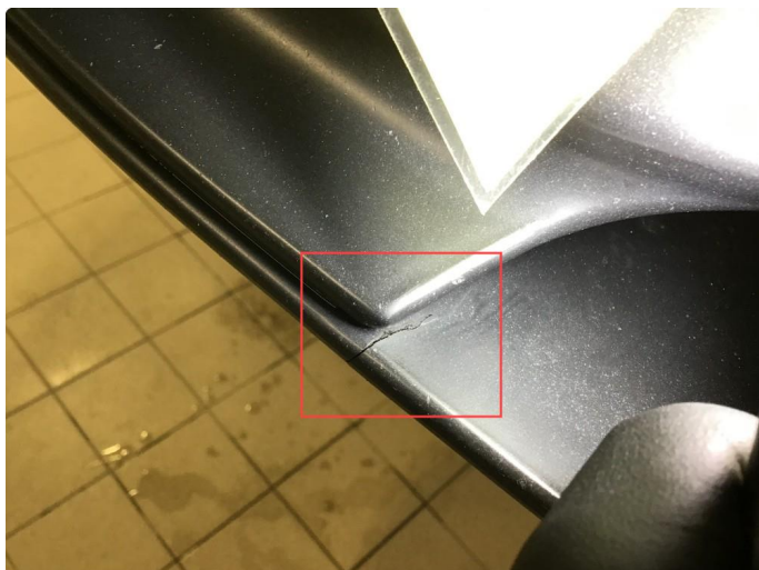
1.5 Liten sprekk i montert frontleppe.
