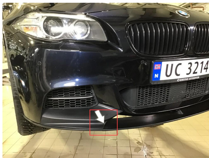
1.5 Liten sprekk i montert frontleppe.
