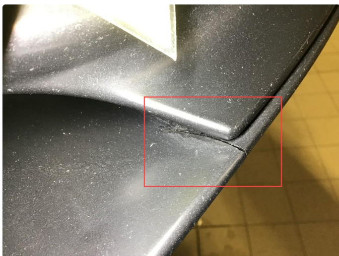
1.5 Liten sprekk i montert frontleppe.
