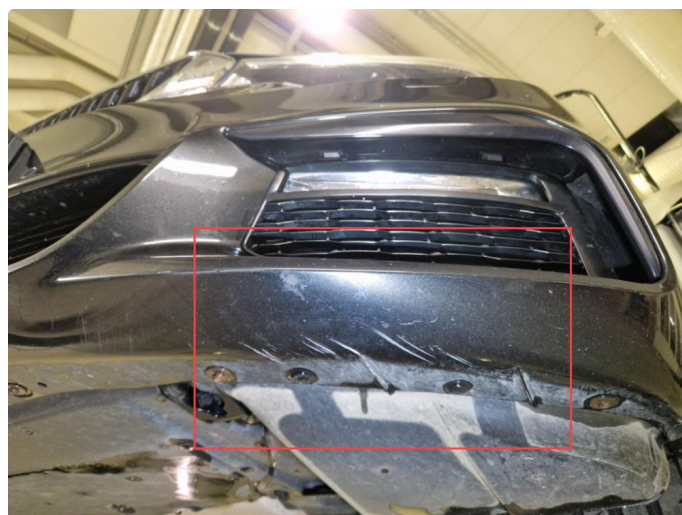
1.4 Noe skrubbskader underside frontfanger .
