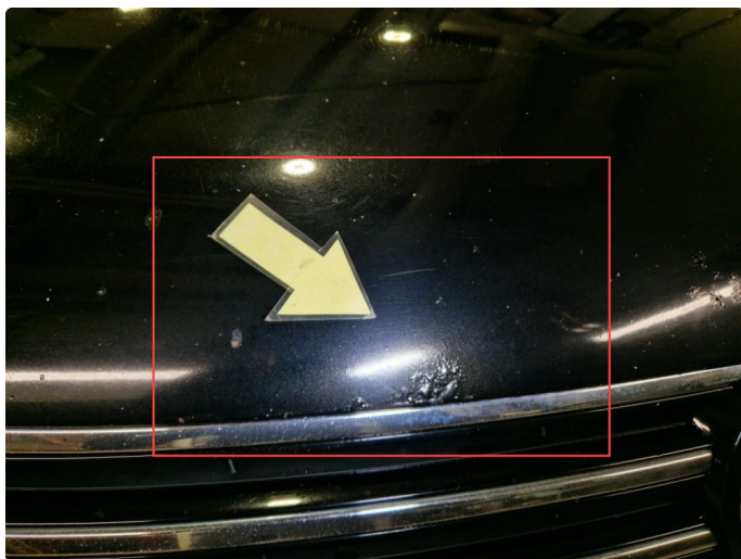
1.2 Rust + mye steinsprut panser.
