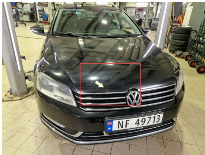
1.2 Rust + mye steinsprut panser.
