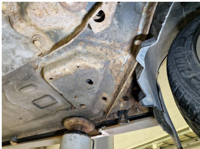
1.1 Rust underside bil.
