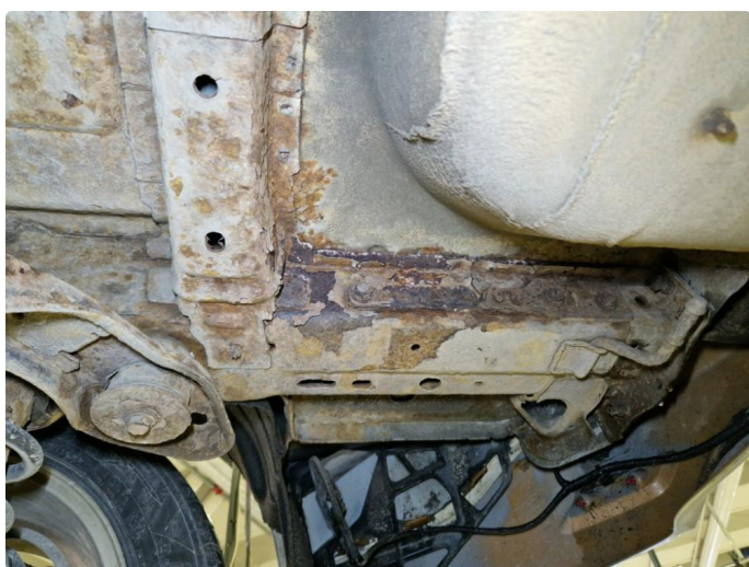
1.1 Rust underside bil.
