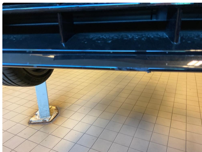
1.2 Spoilerlist defekt (reparert)
