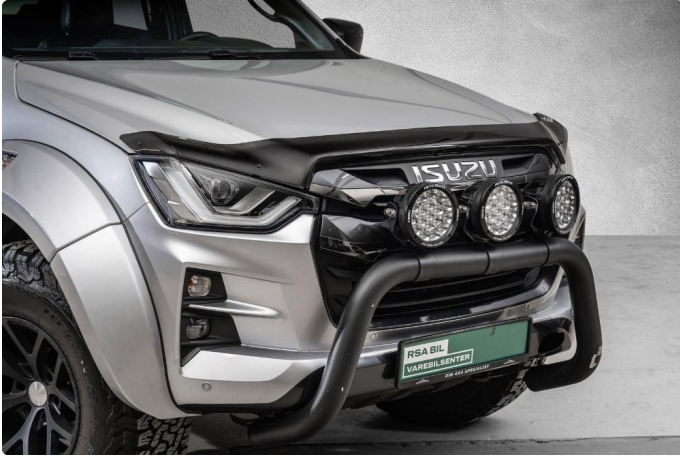
1.1 Steinsprut i front.
