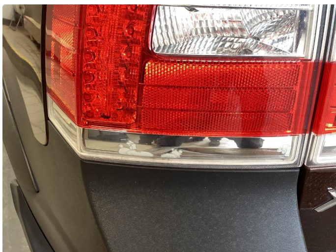
2.1 Krakelering i plast
