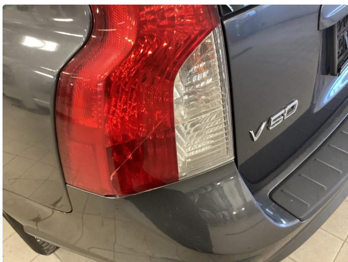
2.2 Defekt / sprukket glass
