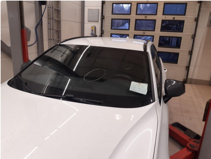
1.1 Steinsprut i synsfelt
