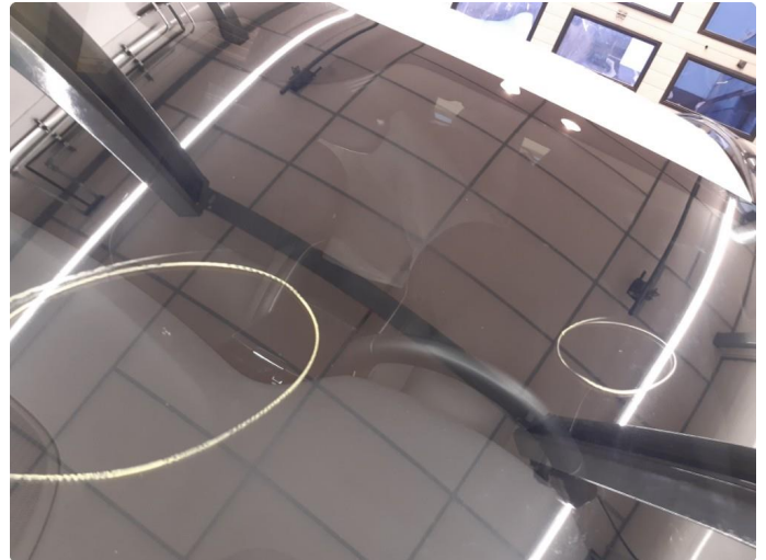
1.1 Steinsprut i synsfelt
