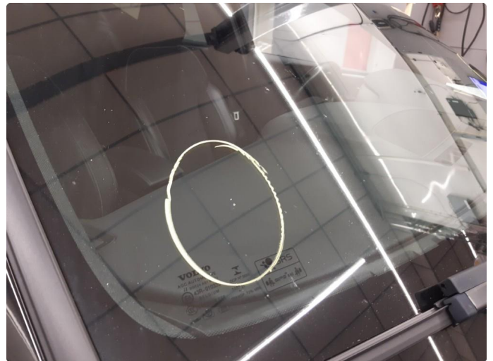
1.1 Steinsprut i synsfelt
