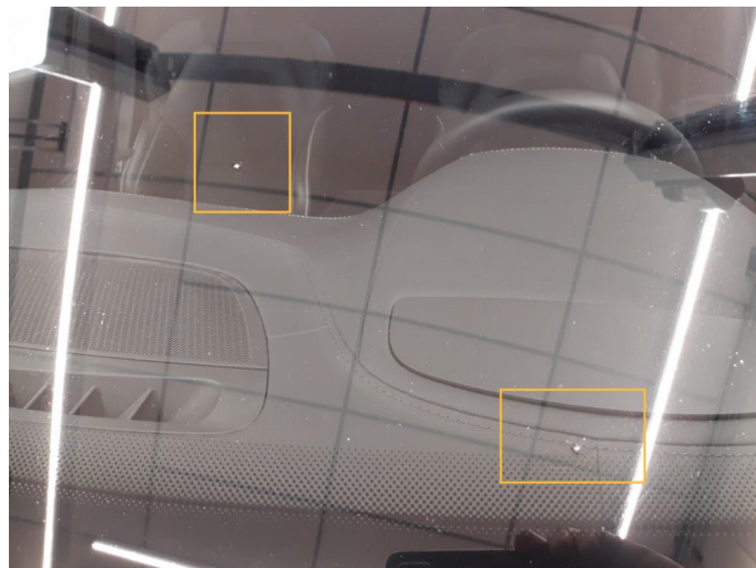
1.2 Steinsprut i synsfelt
