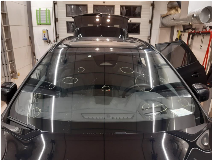
1.1 Steinsprut i synsfelt
