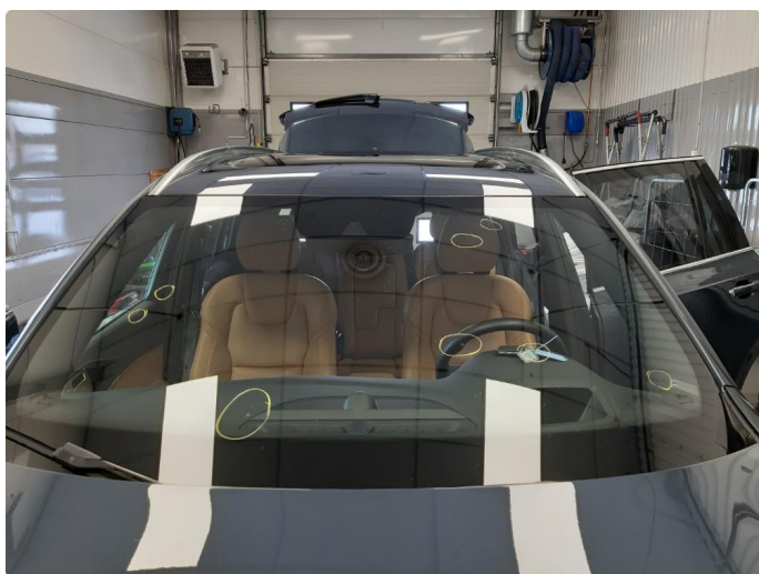
1.11 Steinsprut i synsfelt
