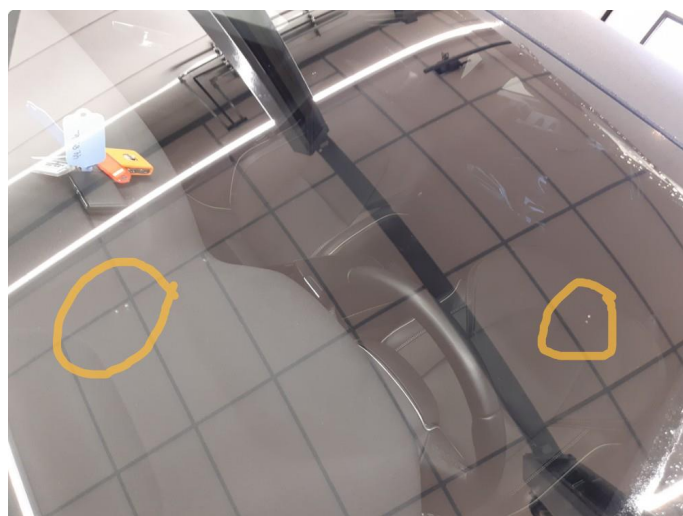
2.2 Steinsprut i synsfelt
