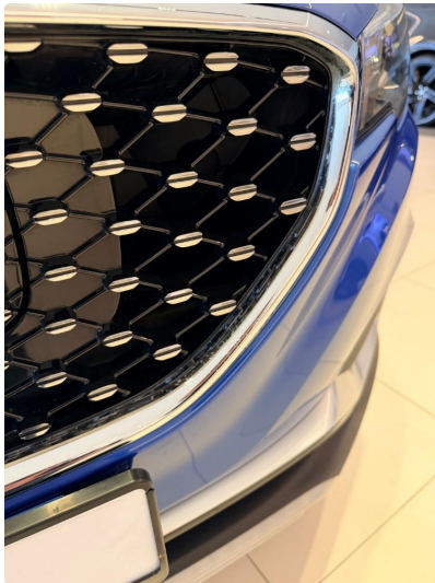
1.3 Krakelering i grill
