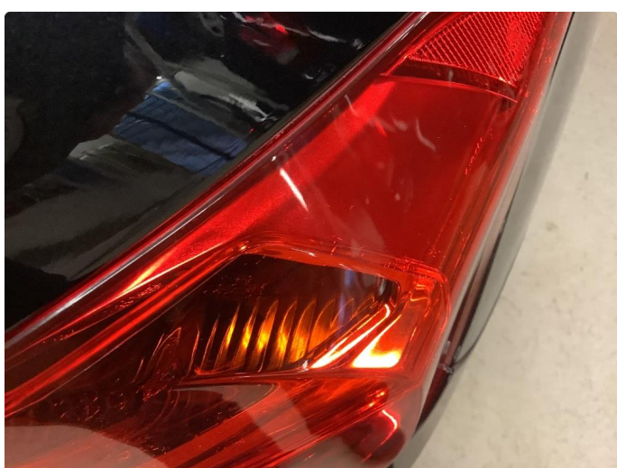
2.1 Krakelering i plast
