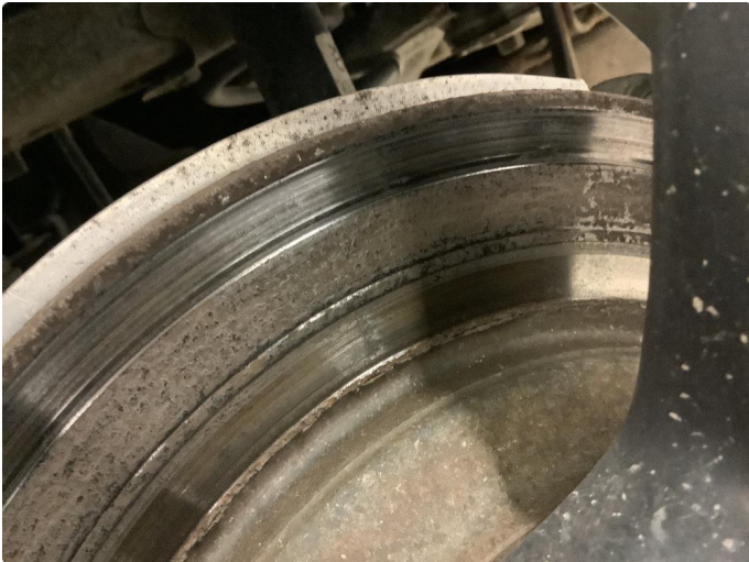
1.1 Mer enn 25% rust
