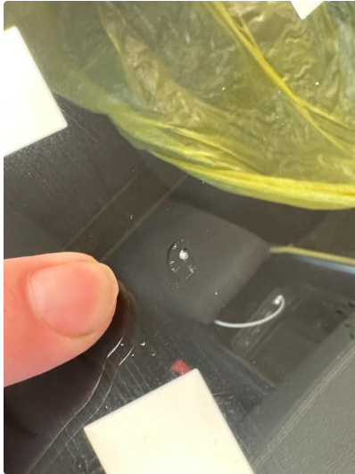
1.1 Steinsprut utenfor synsfelt
