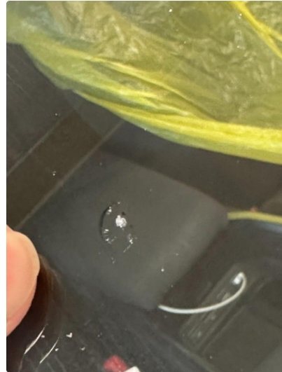
1.1 Steinsprut utenfor synsfelt
