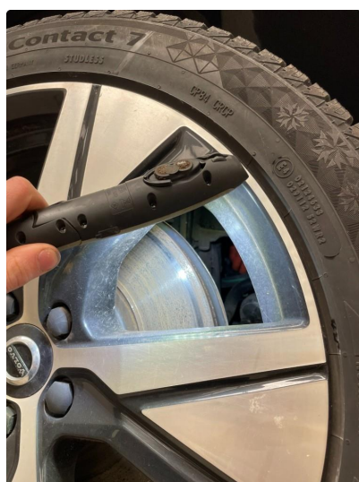
2.1 Mer enn 25% rust
