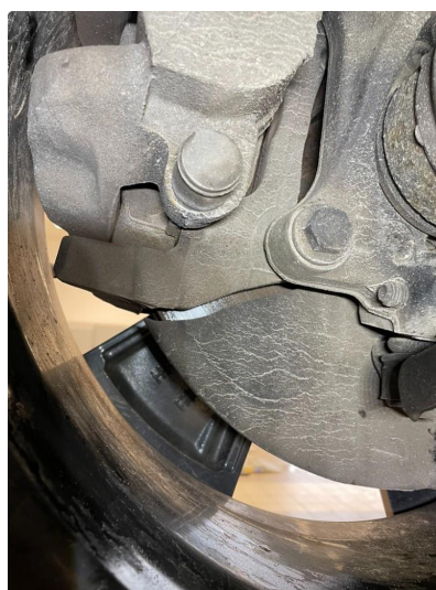
2.1 Mer enn 25% rust
