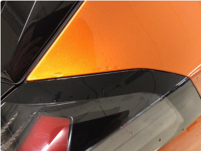
1.1 Krakelering i plast
