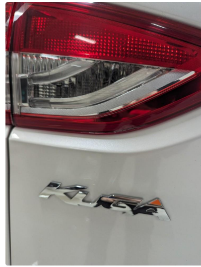
2.1 Krakelering i plast.
