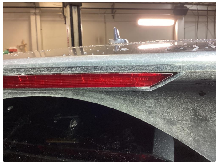
2.2 Defekt / sprukket glass
