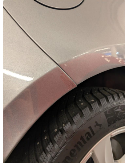
1.2 Lakkavflassing - Penslet i ny lakk.
