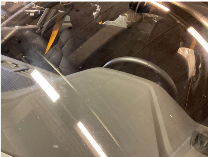
1.4 Steinsprut i synsfelt
