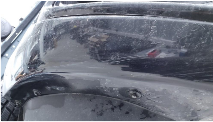
1.1 Riper under frontfanger - Normal slitasje
