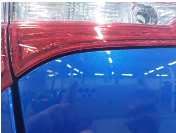
2.1 Krakelering i plast
