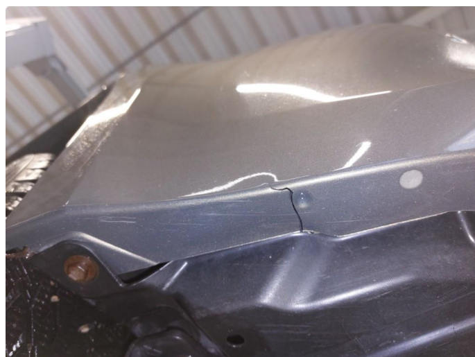
1.2 Liten sprekke under
