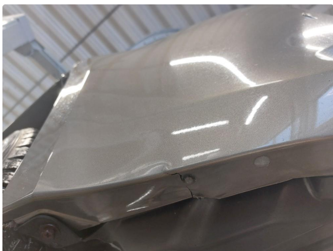
1.2 Liten sprekke under
