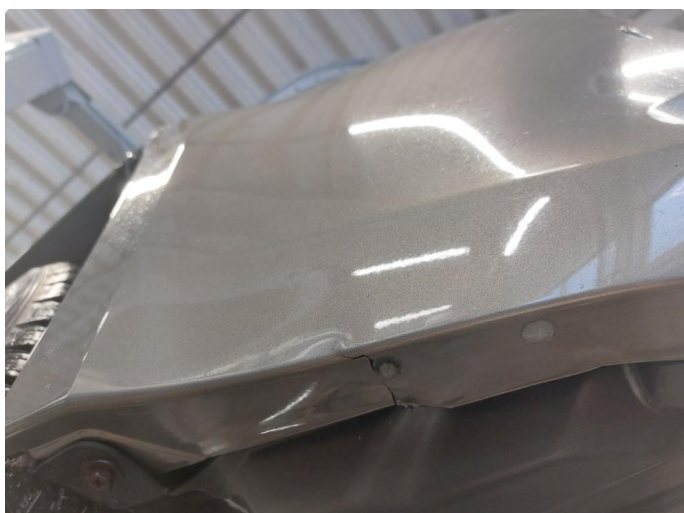
1.2 Liten sprekke under
