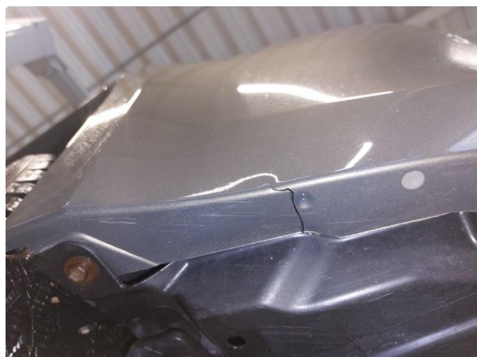
1.2 Liten sprekke under
