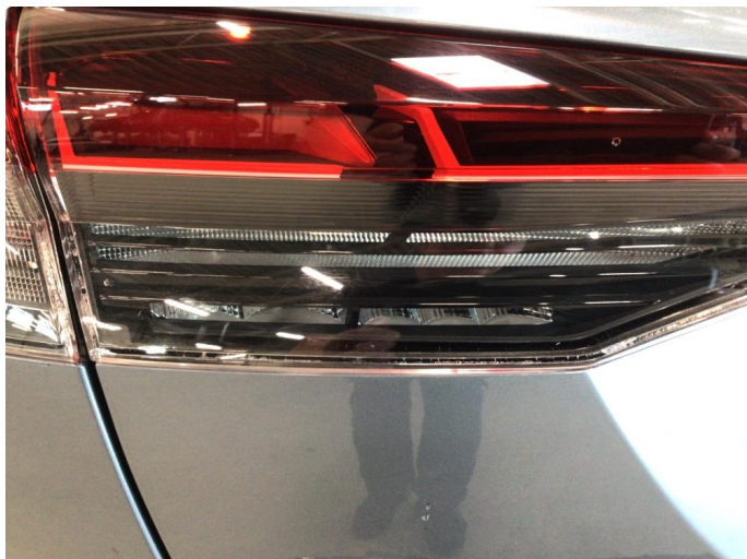
1.1 Krakelering i plast
