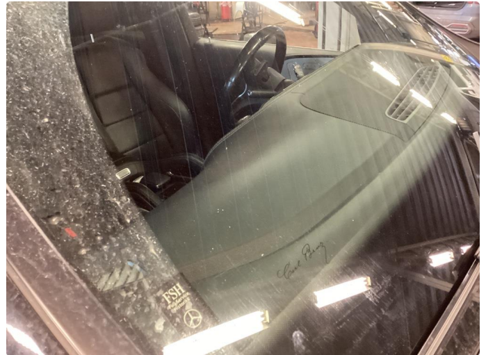
2.2 Steinsprut utenfor synsfelt
