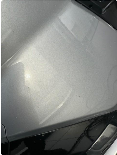
1.1 Steinsprut v.s foran.
