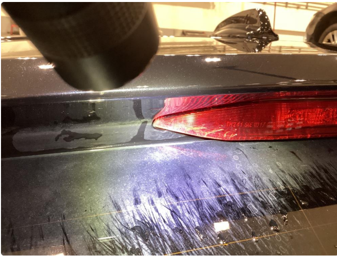
2.1 Krakelering i plast
