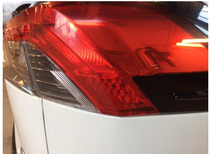
1.1 Krakelering i plast
