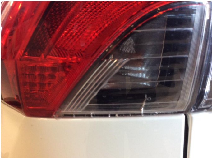
1.1 Krakelering i plast
