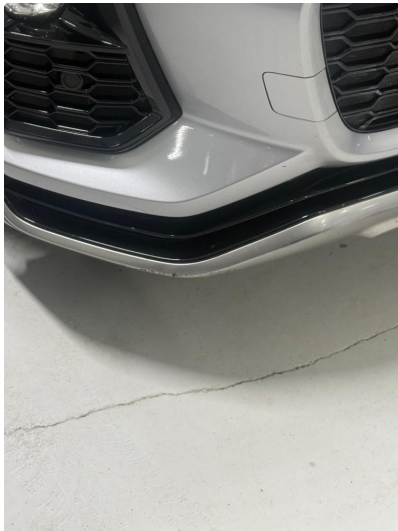
1.1 Spoiler foran - Steinsprut
