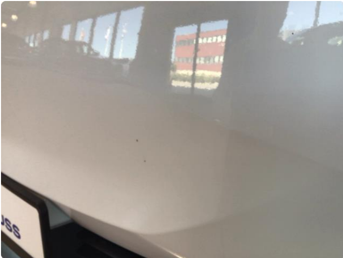
1.1 Liten steinsprut franker front
