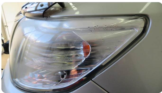
2.1 Dugg/fukt Dugg i lampa.
