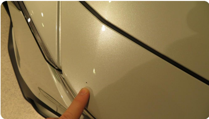
1.1 Steinsprut Liten steinsprut
