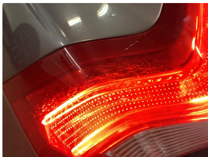
2.1 Krakelering i plast
