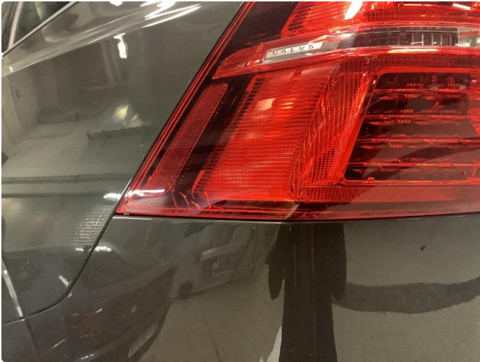
2.1 Krakelering i plast
