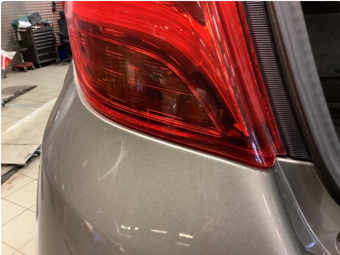
1.1 Krakelering i plast
