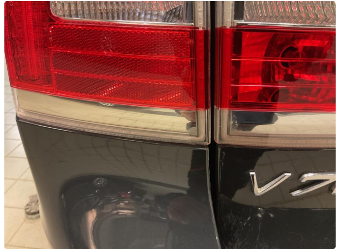
2.1 Krakelering i plast
