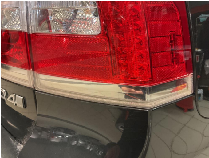
2.1 Krakelering i plast
