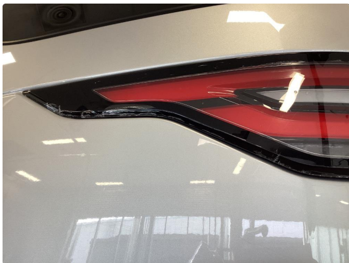
2.1 Krakelering i plast
