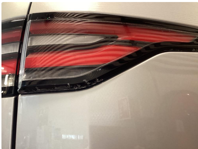
2.1 Krakelering i plast
