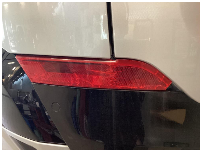
2.1 Krakelering i plast
