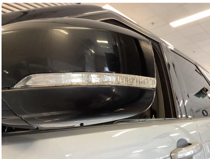
2.1 Krakelering i plast
