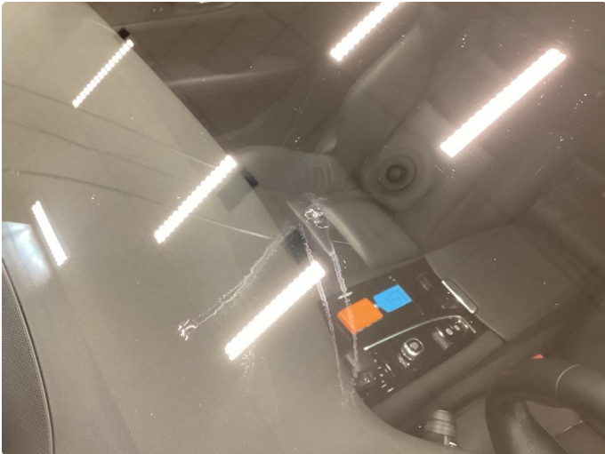
1.1 Steinsprut utenfor synsfelt/repareert
