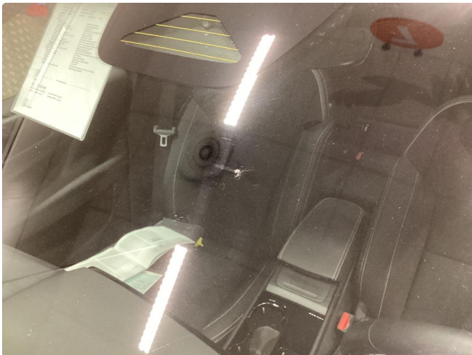
1.3 Steinsprut i synsfelt
