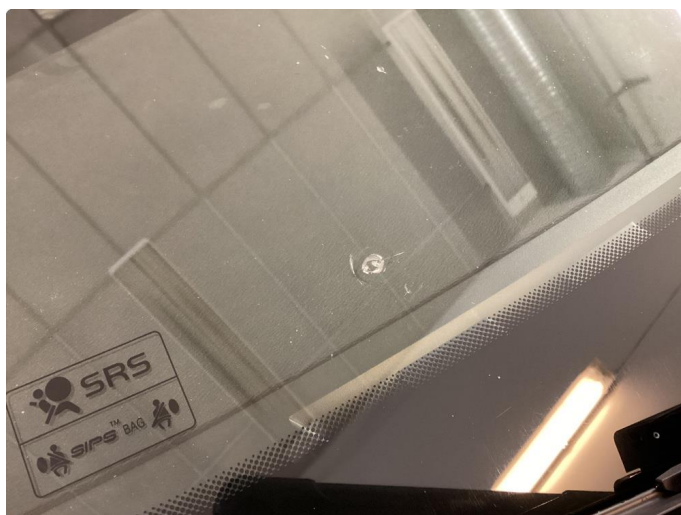
1.2 Steinsprut utenfor synsfelt
