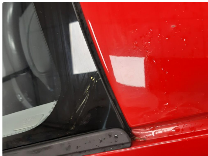
2.8 Steinsprut i synsfelt
