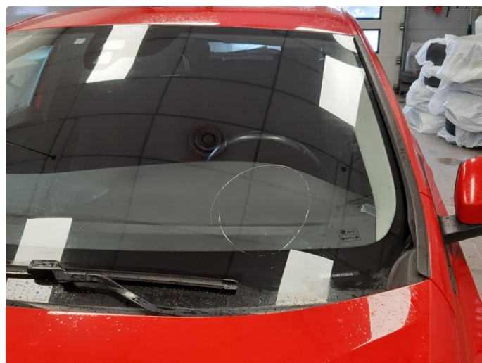
2.8 Steinsprut i synsfelt
