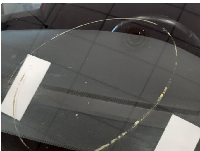
2.8 Steinsprut i synsfelt
